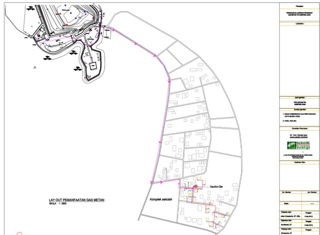
Fig. 2.1-27. Methane Harvesting Network Plan of Gampong Jawa Sanitary Landfill Source: Environmental, Sanitation, and Beautification Authority of Banda Aceh (Dinas Lingkungan Hidup, Kebersihan dan Keindahan Kota), 2018
